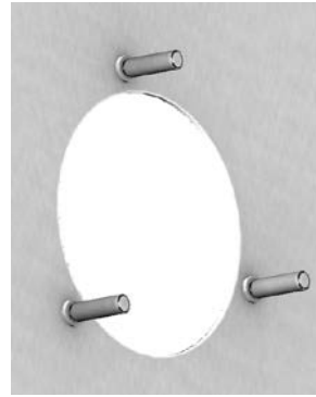
Example for housing with screws from the panel front for mounting without mounting ring
