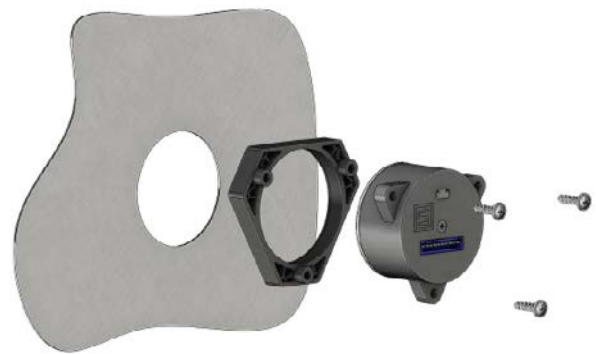
Mounting of the Design-In-Kit using the mounting ring
